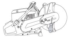
When a diamond blade is mounted on the power cutter make sure that the diamond blade will rotate in the direction indicated by the arrow on the blade.
